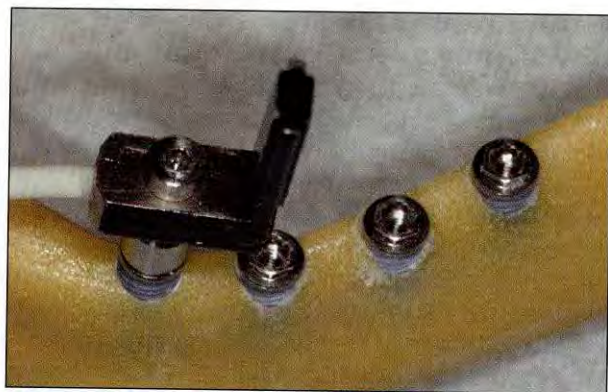
Fig 1a An Osstell transducer attached to a regular-platform (RP) Brånemark System implant parallel to the alveolar ridge of a synthetic bone model.
